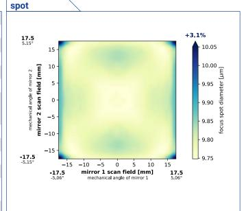
spot diameter at 86.5% level for a Gaussian beam ( $M^2 = 1$ ) with 10.0 mm diameter at 1/e2, clipped at 10.0 mm field size and mirror distances as given above for a two mirror scan system
