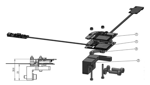
Figure 11: Mechanical layout of the LSR-4C-LL (double diffusor with bracket) assembly: (1) LSR-4C, (2) Bracket kit LSR-4, (3) LSR-4C-LL-mounting kit.
