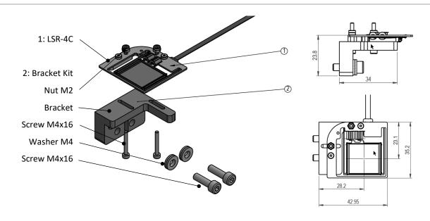
Figure 10: Mechanical layout of the LSR-4C-L (with bracket) assembly. The LSR-4C is mounted onto the bracket which can then be mounted into an existing setup. The weight of the bracket is 43 g.
