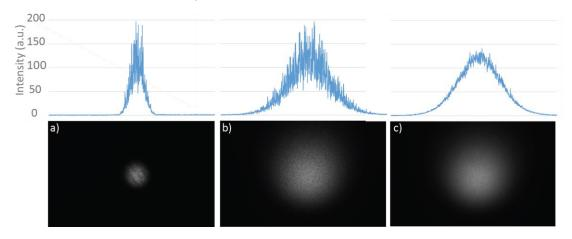
Figure 1: a) shows the intensity distribution of the bare laser beam with a wavelength of 532nm. The speckle contrast C is 0.27. In b) the LSR is placed in the beam path but turned off and the speckle contrast is 0.26. In c) the LSR is oscillating, reducing the speckle contrast to 0.06.
