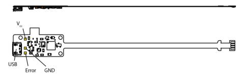
Figure 8: Pinout of the flex electronic. Power can be supplied via the micro-USB connector or the soldering pads.
