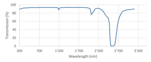
Figure 5: Transmission spectrum of the LSR-4C with the uncoated standard diffusor.
