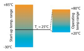
Figure 3: Graphical illustration of the final operating temperature range based on a start-up temperature of  $25^{\circ}$ C.
