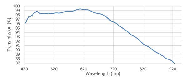
Figure 4: Transmission spectrum of the LSR-4C with the coated standard diffusor.
